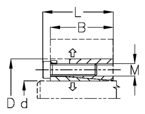
$\begin{array}{lll} \text{B mm} & = 44.0 \\ \text{d H8 mm} & = 110 \\ \text{D mm} & = 155 \\ \text{Fit tolerance} & = \text{Aksel h8, Nav H8} \\ \text{F kN torque} & = 260 \\ \text{L mm} & = 56 \\ \text{M mm} & = \text{M12} \\ \text{P N/mm2 surface pressure on shaft/hub} = 160 \\ \end{array}$
